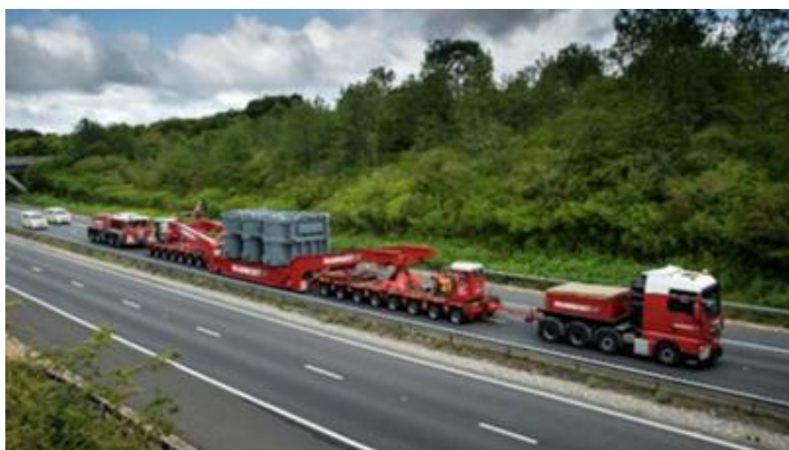
Image 5.23 Illustrative Abnormal Indivisible Load delivery vehicle
